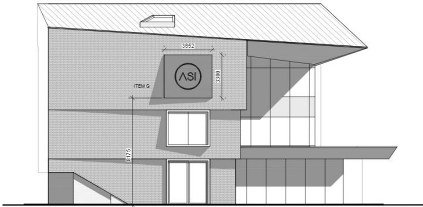
Sign I High level lettering on side of hangar covering a total area of 8.81m x 2.05m (internally illuminated white letters):
