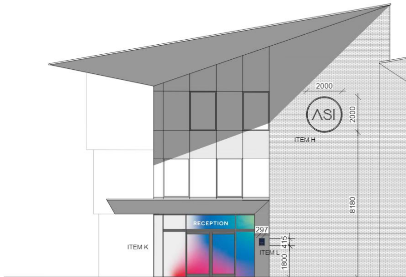
Sign K Reception vinyl applied internally to glazing, Sign L 0.296m x 0.429m acrylic wall mounted panel and Sign H 2m x 2m high level circular wall sign (internally illuminated/white)
